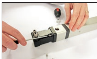
Tighten motor mounting screws
