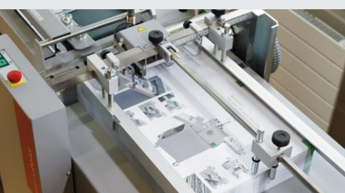
Paper feeder for folding machine
