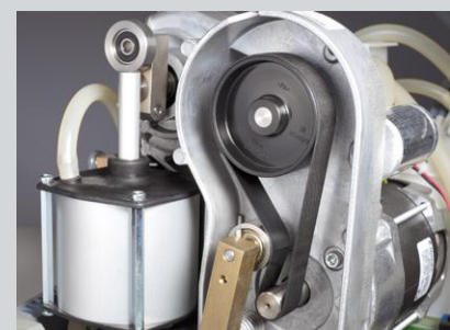
Flat belt drive of a suction pump
