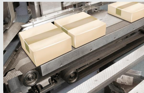
Accumulating conveyor belt for carton
