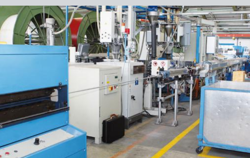
Extrusion plant for tubes FDA approved
