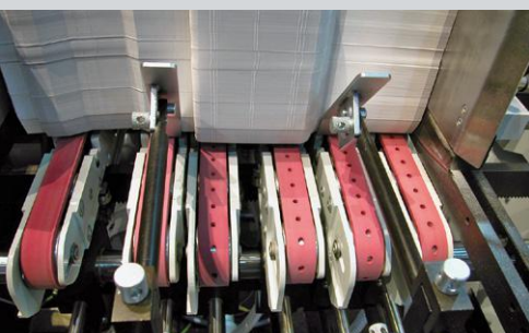
Feeder unit of a folder/gluer machine
