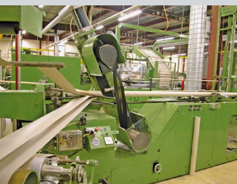
Tube winder belt 565 TW, 3150x120x4.0 mm
