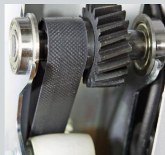
Drive for friction rollers
