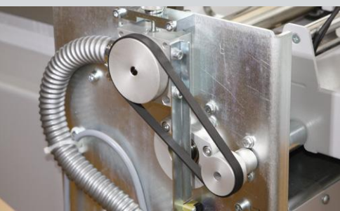
Light power transmission of paper drive axle
