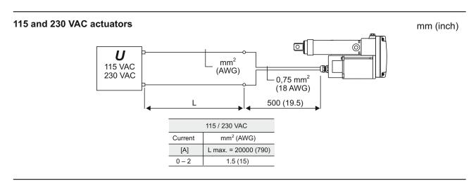
Always install fuse and / or thermal breaker between motor and power supply to protect actuator, wiring and other items.
