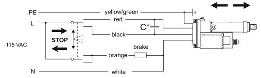
\* A capacitor must be installed to between the motor windings to able to run the actuator. 115 VAC actuator = 25 microF, p/n 5704687, 230 VAC actuator = 6 microF, p/n 7825261.
