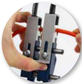
Quick clamp device for inserting the profiles in exchangeable profile jaws.
