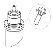
The motor flange must be tightly fitted onto the gearbox. Screws with a strength class of A4-70 must be secured. Tightening torque ( $T_{A,S}$ ) of the screw is 90% of screw yield strength. Tighten screws crosswise with  $T_{A,S}$ .
