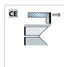
Bellows outer collar. Suitable for screw fastening.
